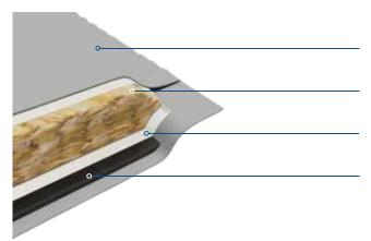
PVC fabric with fibreglass (0.18 kg/m²)
