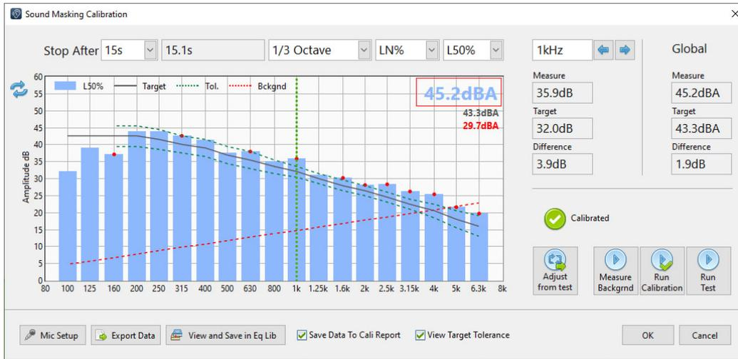
If no red points are showing, it means that tolerance conformity is validated.
