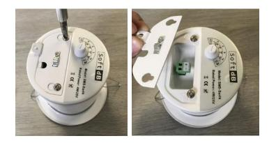
2) Pass the power wire(s) through the wire guide lock and connect the wires in the green terminal block.
